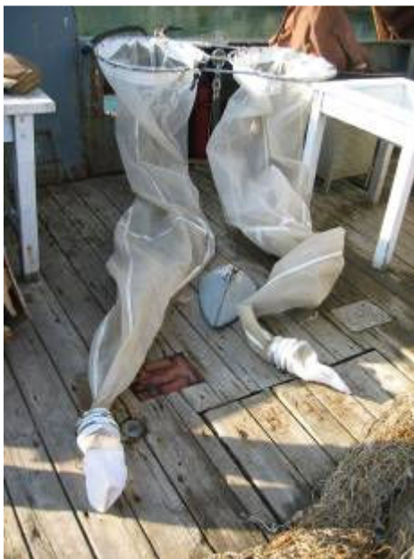
Figure 23 Bongo net for ichthyoplankton sampling
