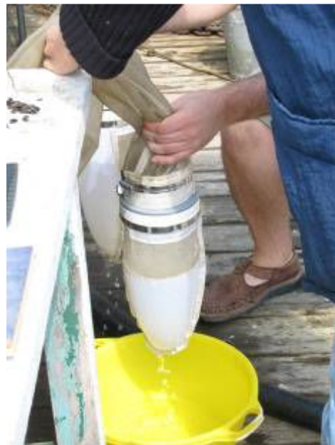
Figure 23 Bongo net for ichthyoplankton sampling
