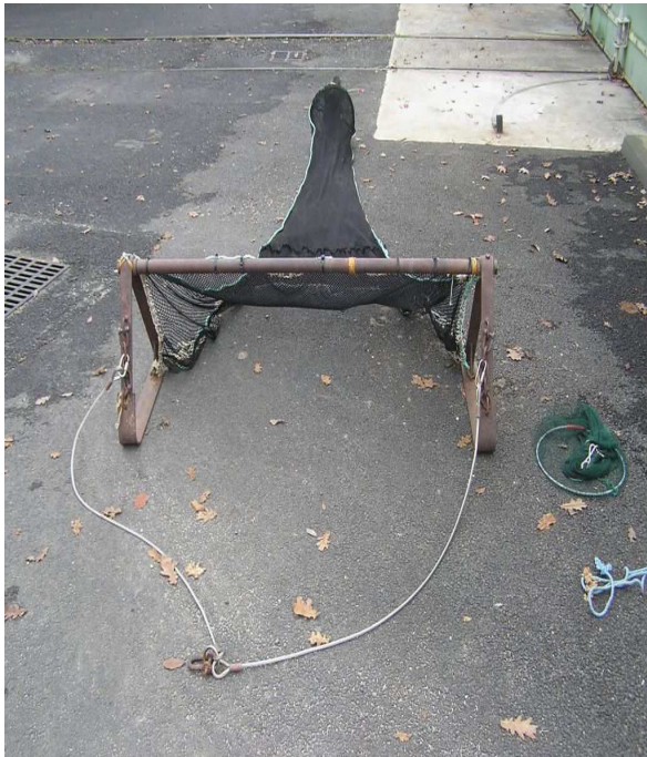
Figure 8 A. Beam trawl
