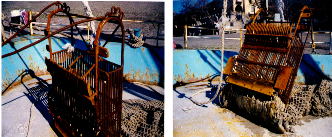
Figure 11 Metallic dredge for baby clam extraction from soft ground (A, B).
